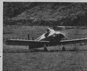
A home made plane, powered by a VW engine
